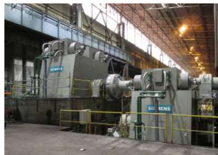
Giant motors of 12 MW at Châtelet..
