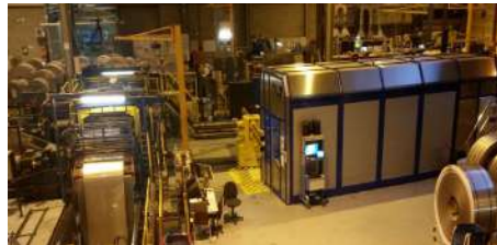
Automatic system for slitting lines at S&S Germany (Sersheim).
