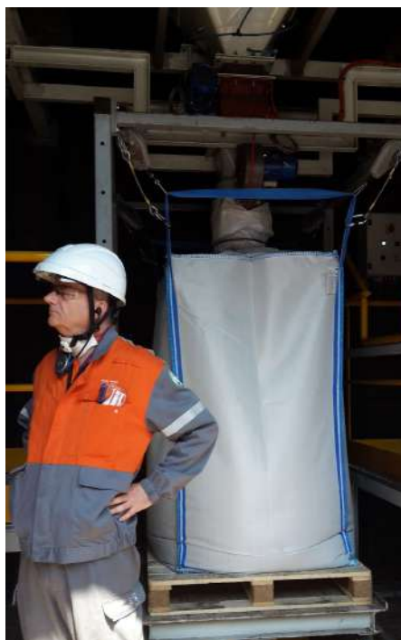
Imphy melting shop: recovery of the dust in bags ready to be sent to Recyco.
