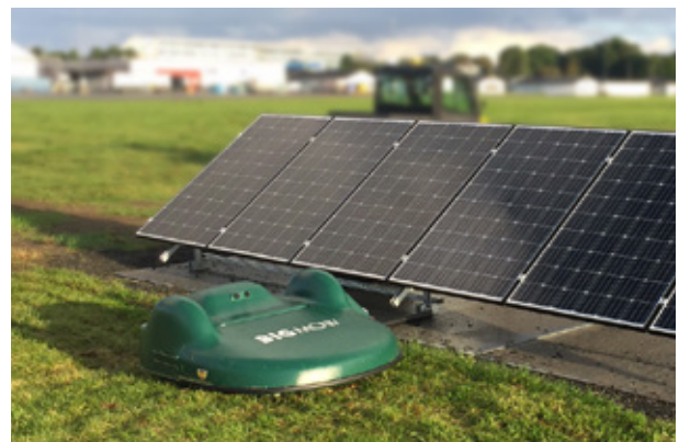
In Stavanger 16 electric robotic mowers charged by solar panels helped to keep the grass cut in the summer. The solar panels and batteries help to ensure that the mowers always have power. They have a capacity of 20 square kilometres, which is necessary along the 2.5-kilometre-long main runway.
