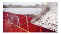
After harvesting, the cranberries are pumped onto a vibrating conveyor and loaded onto a truck.
