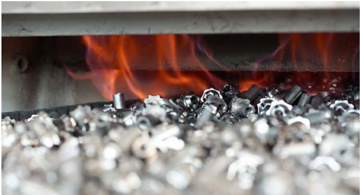
The new heat treatment system, now equipped with low-emission flameless oxidation (FLOX) burners, reduces CO 2 emissions.
