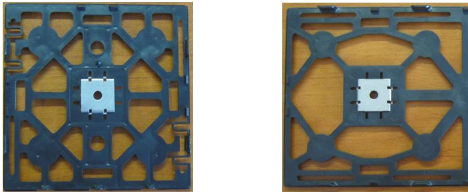
The example above illustrates the plastic gain that can be achieved on a part. In this example, DIAM achieved a material gain of 21%.
