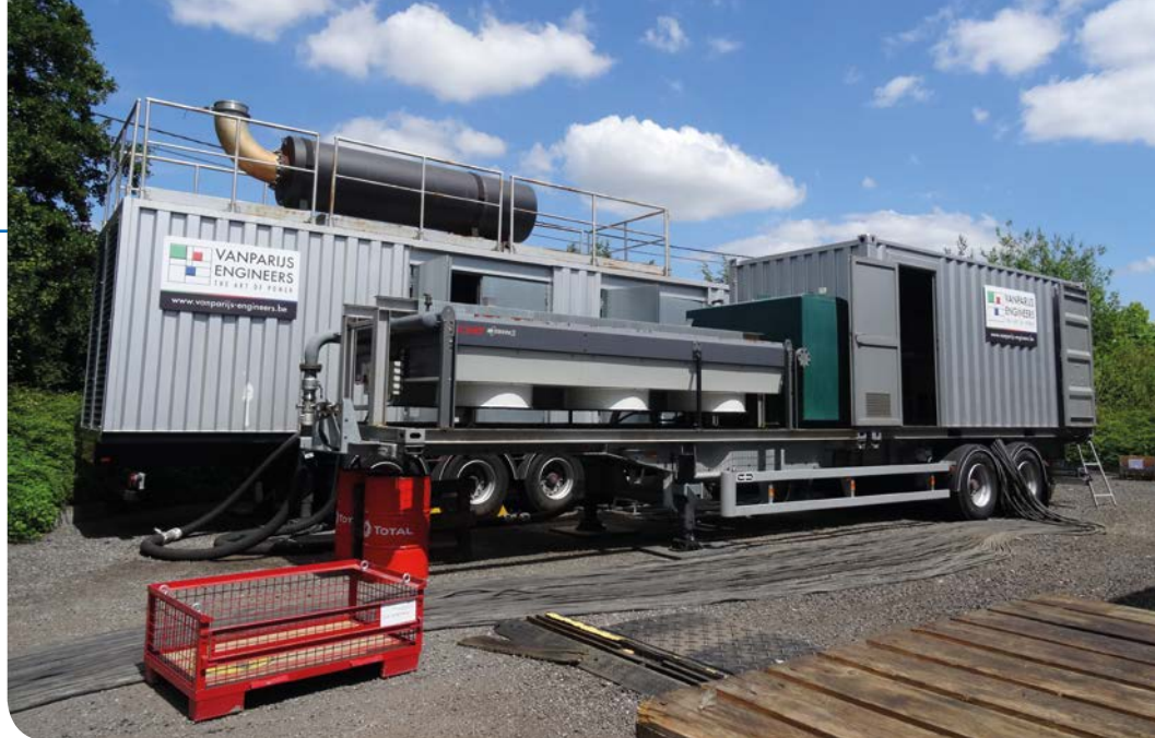
This mobile, uninterruptible power supply unit is the most powerful in Europe. Owned by of Vanparijs Engineers, it is leased to IT centres, airports, pharmaceutical factories, etc., which cannot risk micro-power cuts.
