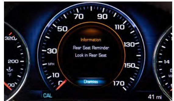
The new Rear Seat Reminder uses audio and visual cues to prompt drivers to check their back seat for passengers, such as children or pets.
