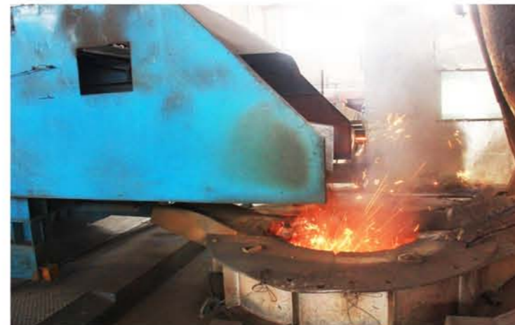
Smelt the iron materials like foundry returns with electric furnace for reutilization.
