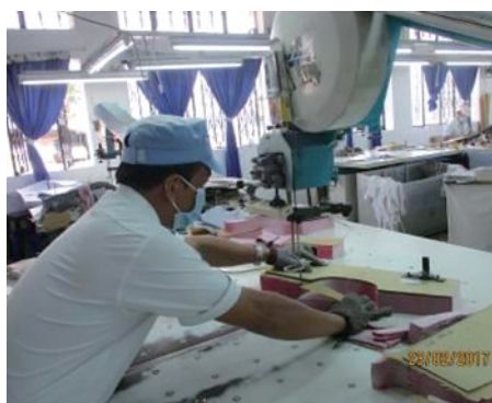
Wearing appropriate personal protective gear when cutting fabric
