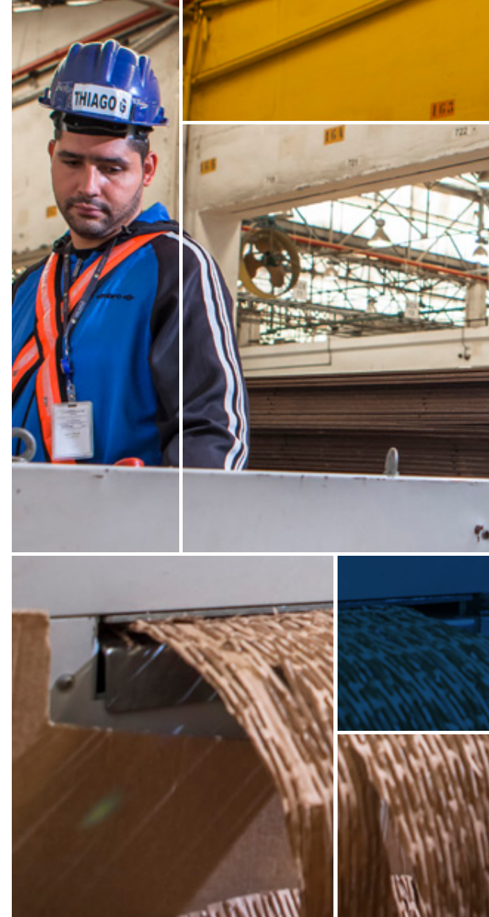
Reutilization of the carton packaging at the São Paulo Unit, transforming them into a mesh that is used to transport parts.
