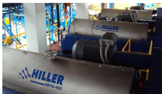
Waste water treatment systems using direct dehydration technology are employed in all fishmeal plants in Copeinca, one of our Peruvian subsidiaries
