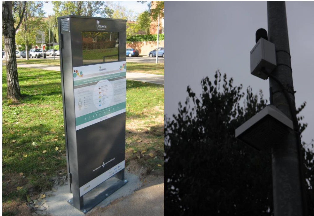
LIQUENS panel and the noise sensor CESVA TA120
