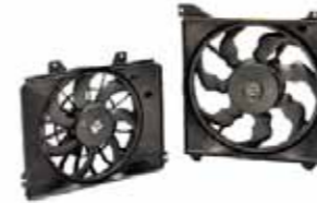
Fan and shroud made of recycled PA
