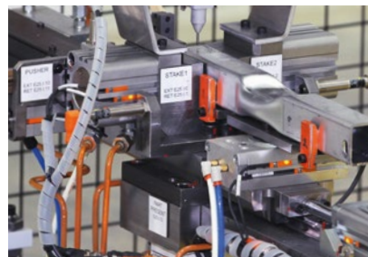
Crash boxes are made on a fully automated production line to ensure precision.
