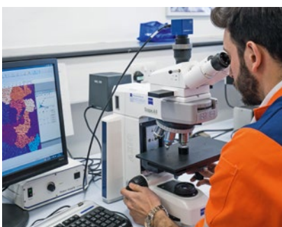
A Constellium research fellow examines the microstructure of an aluminium alloy.
