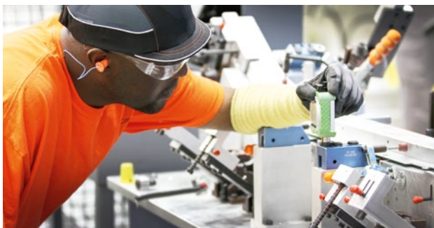
An operator performs a quality check on an aluminium bumper beam.
