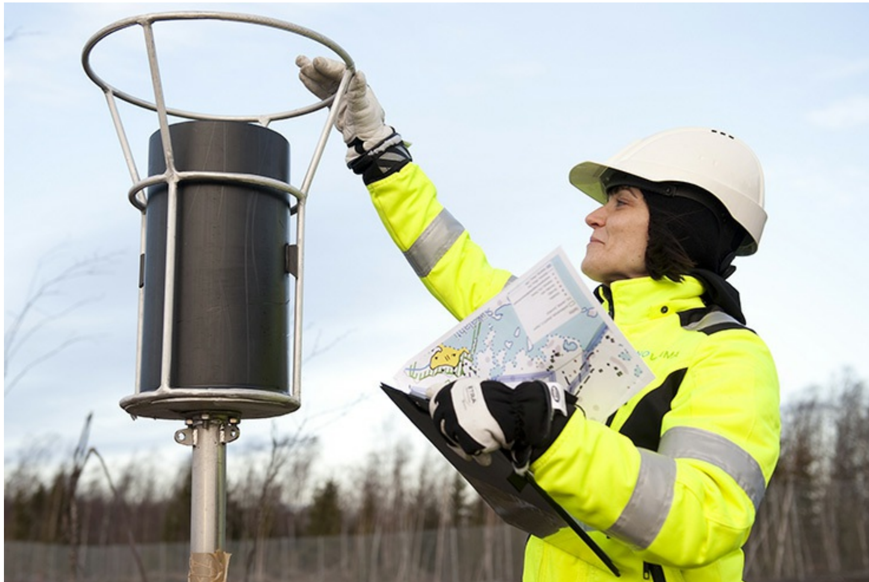
Dust is one of the environmental impacts of construction. Dust is continuously measured at Hanhikivi headland. Photo: Jarmo Tyyskä
