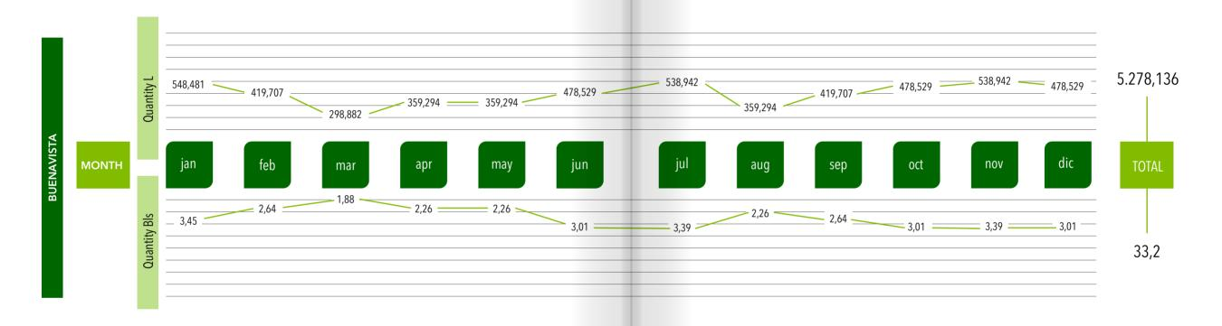
Increase in production water discharge of Buenavista Block related to 2014 corresponds to the behavior of the deposits of some wells that reflected an increase in the water cut and due to the drilling in Santander Sur, because this was a new project that was developed in 2015.
