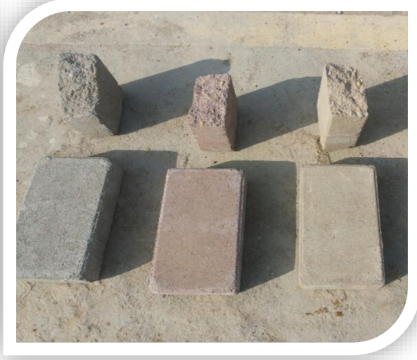
Bricks manufacturing by Effluent Treatment Plant Sludge
