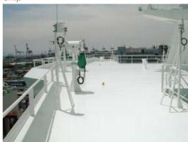
On this ship, ZEFFLE helps prevent salt corrosion, keep temperatures down, and maintain the appearance
