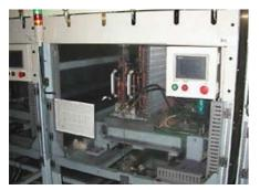
1. Air-tightness and pressure resistance inspection
