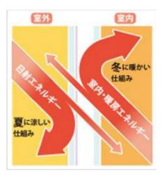
Thermal insulation using low-E glass
