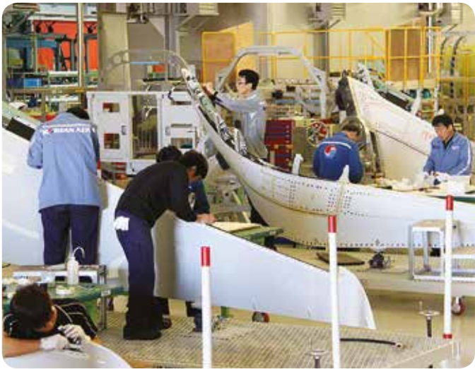
Mechanics working at the final stage of assembling the sharklets for the A320
