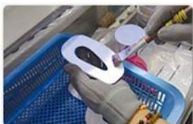
Before Using Cold Fusion Bond midsole part with primer and cement
