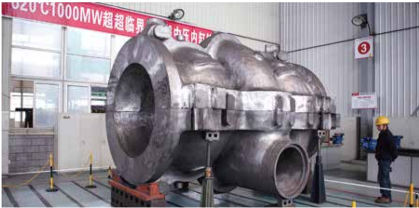
The first 620°C1000MW ultra supercritical steam turbine cylinder casting in the world
