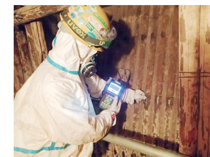
Measuring the thickness of boiler water tubes
