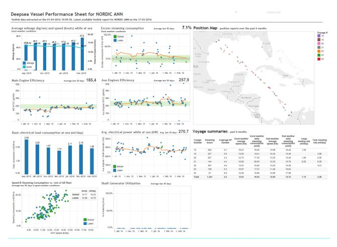
This new vessel performance program also makes it possible to calculate the transport work and energy efficiency, EEOI (tons CO2/(tons cargo x nautical miles)) for our fleet. These data are reported to the Danish Ship owner's Association and will make basis for our EU MRV (Monitoring Reporting and Verification) reporting which will become a requirement from 2018.
