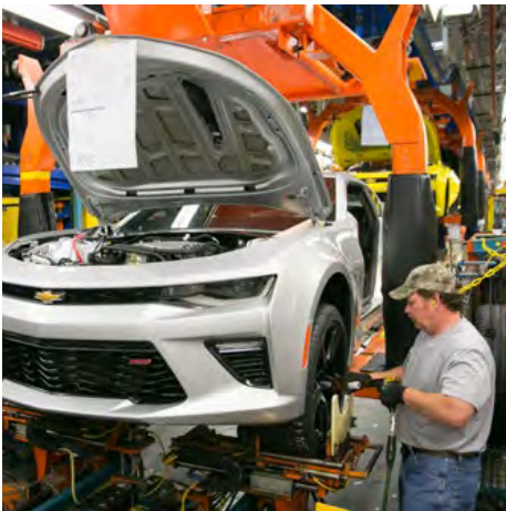
GM employee installs wheels and tires on a pre-production 2016 Chevrolet Camaro for testing.
