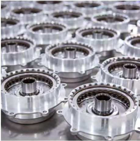
All-new Chevrolet Volt drive units await final assembly.
