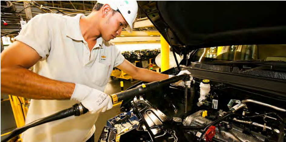
An employee in the General Assembly shop at GM's Rayong, Thailand, manufacturing plant during engine installation
