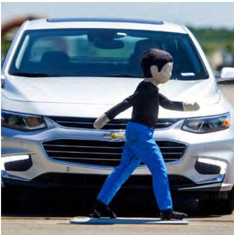
Front Pedestrian Braking, a new active safety technology available on the 2016 Chevrolet Malibu and 2016 Cadillac CT6, is one of many safety features tested at our new Active Safety Test Area at the Milford Proving Ground.
