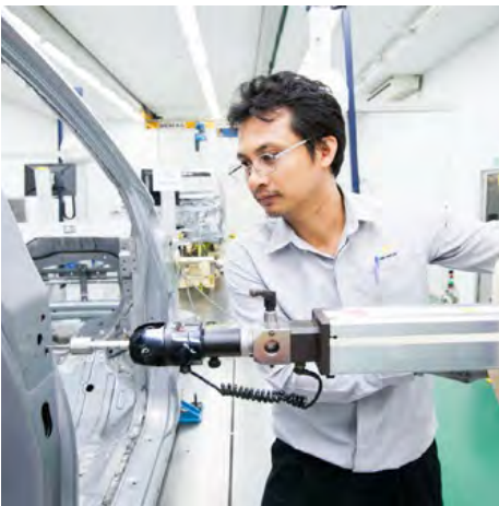
An employee in the Body Shop of GM's manufacturing plant in Rayong, Thailand, takes precise digital measurements of a Chevrolet Captiva's supportive structure to ensure the body parts are accurately assembled.
