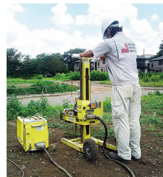
Housing site ground inspection by screwdriver sounding test
