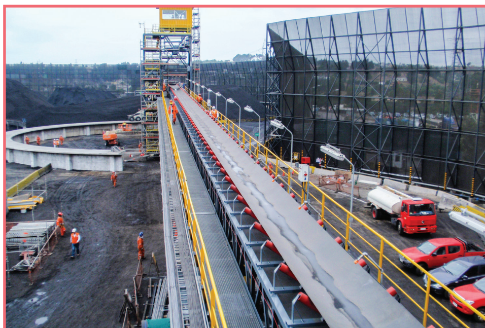
Rubber Belt Conveyor for bulk materials transportation
