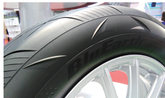
Adding protruding fins to the side wall of the tire helps to control airflow
