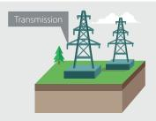
Transmission companies are the Group companies that transport energy via transmission towers and transformers (structures known as the Basic Network) from the plant where it is generated to the distribution substations from where it is distributed to end consumers.
