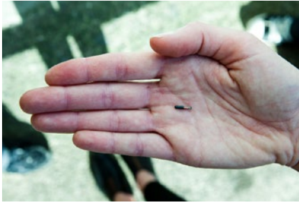
Chip which is implanted into the eels. It sends a signal to migromat when eels start to migrate. Running of the landside turbine can be reduced and blades can be opened as wide as possible in order to facilitate migration.
