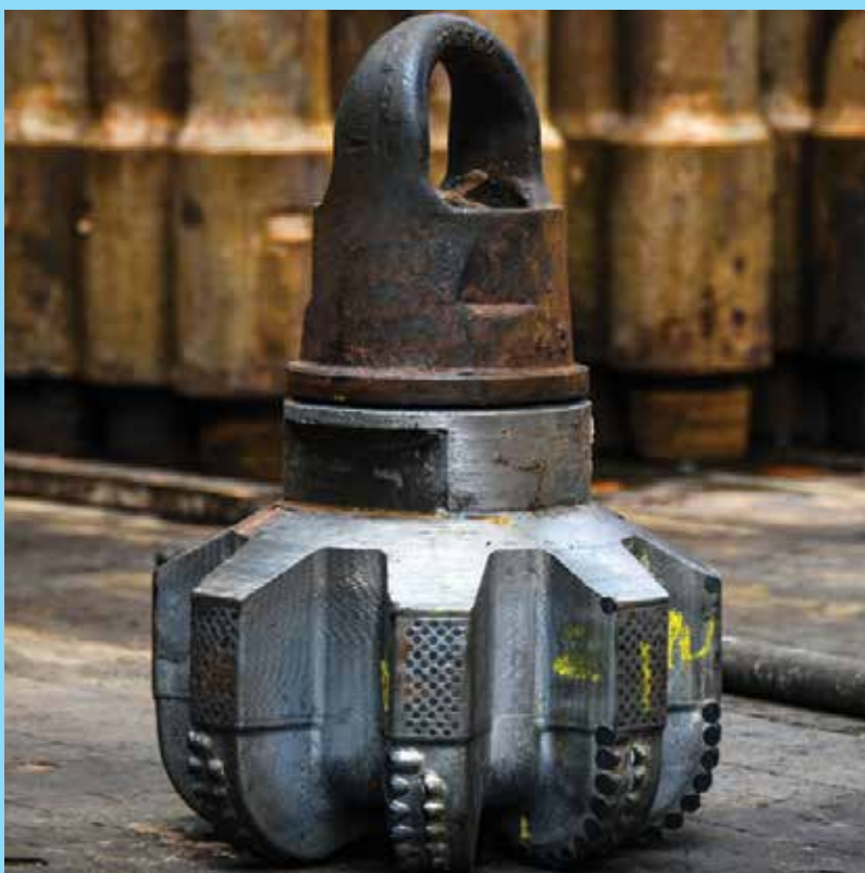
A used drill bit on the drilling floor of the Atwood Achiever while on location offshore Senegal.
