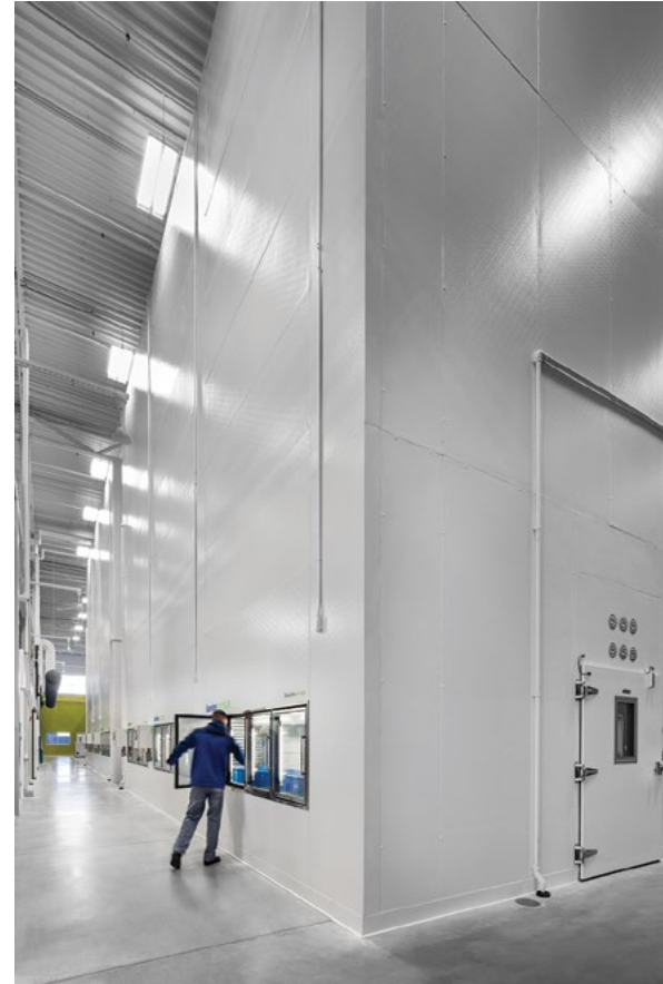
Vertical lift modules for cold-chain storage optimize efficiency and reduce loss of treated air in freezers
