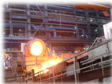
Liquid ferronickel granulation
