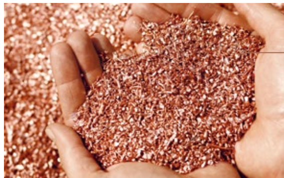
Copper granules recovered from cable waste by Aurubis' subsidiary Cablo
