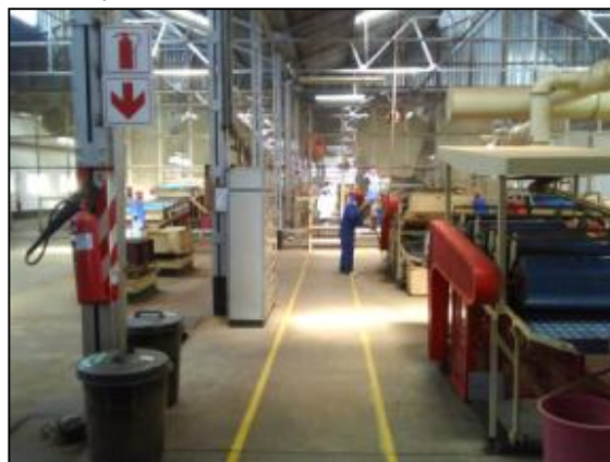
Photo 8: Inside one of the factories. Note the housekeeping, marked walkways, guarded machinery and fire extinguishers provision.
