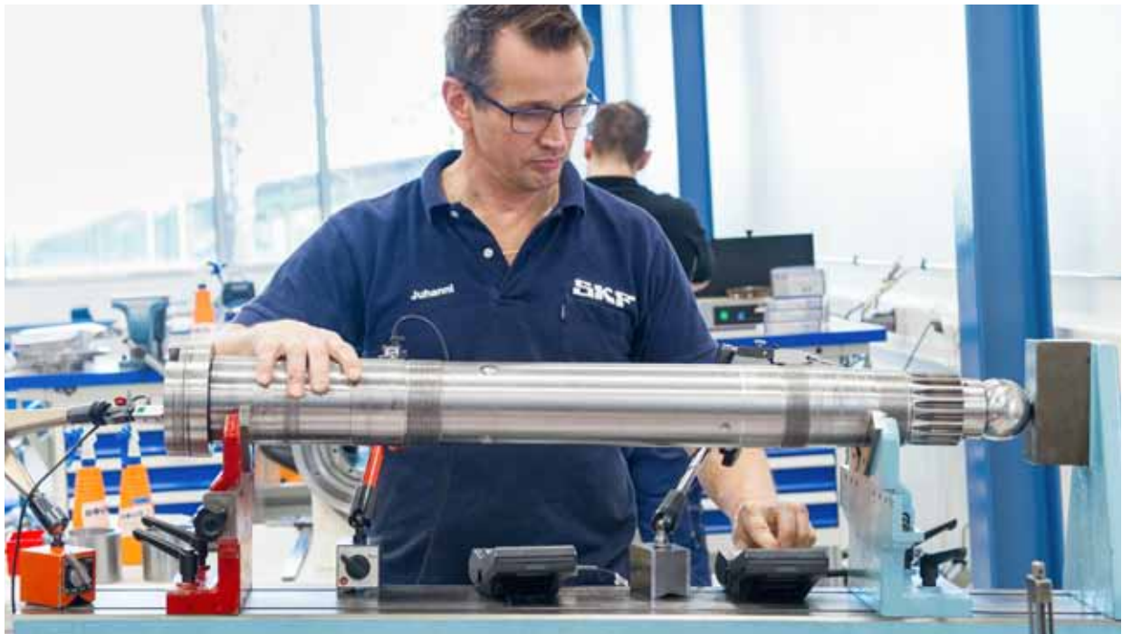
Juhani Knuuti, Spindle service at SKF Solution Factory in Gothenburg. In this picture, the shaft of the spindle is checked to decide if any repairs are required.
