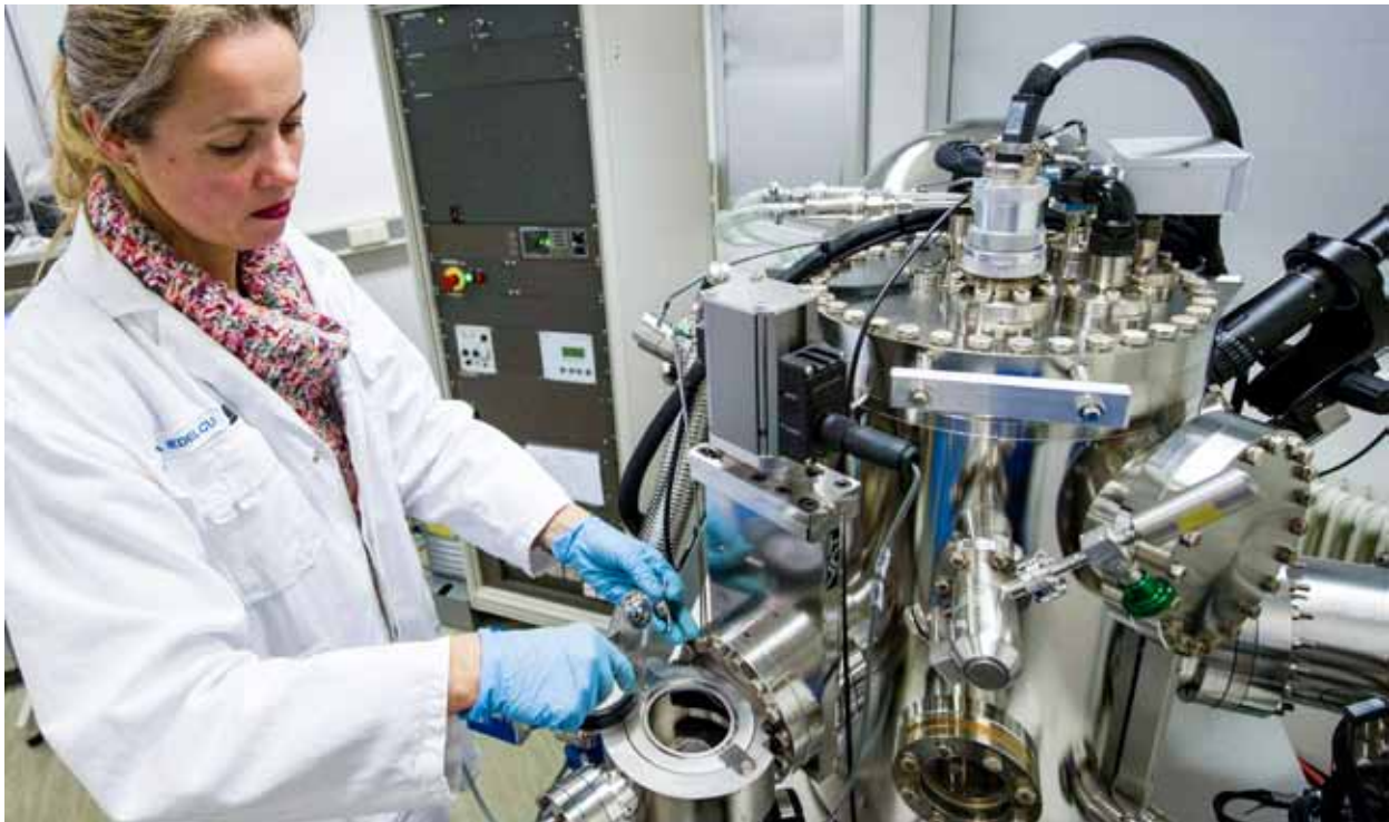
Ileana Nedelcu, Researcher, Tribology and Lubrication Department, is analyzing the surface chemical properties of the raceway of a bearing using XPS (X-ray Photoelectron Spectroscopy). This is to be able to study the impact of the additives of the lubricant on wear and surface life.
