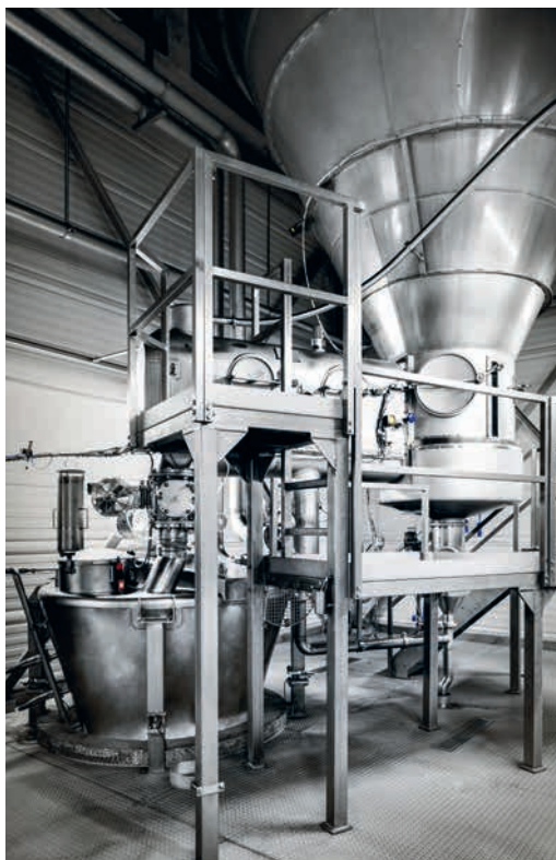
In the spraying tower, the flavor compositions with various carriers are fed into an airstream heated to 190 degrees Celsius. There they dry to tiny particles within seconds. The flavors are encapsulated that way, can be dissolved easily in the finished products and have an extremely long shelf life.
