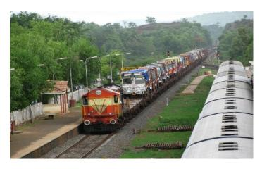
Konkan Railways' novel experiment initiated on 26.01.1999 with `Roll-on Roll-off' of trucks over BRN wagons has been a resounding success. Introduction of Roll On - Roll Off services has been a WIN-WIN situation for Railways, Road Transporters as well as to the Nation. One to two hours of terminal detention coupled with 100% loaded traffic in both directions has resulted in better financial returns for Railways.
