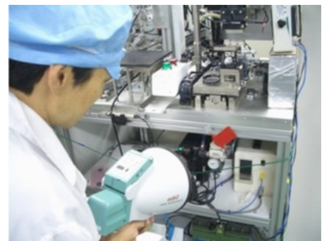
Measuring air leaks at points marked with arrows
