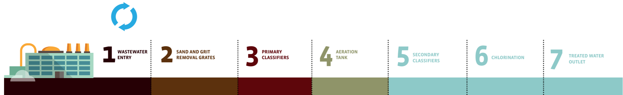
SEWAGE DECONTAMINATION PROCESS
