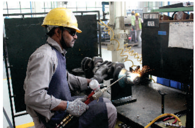
Metal spraying- one of the reconditioning approaches at Prolife
