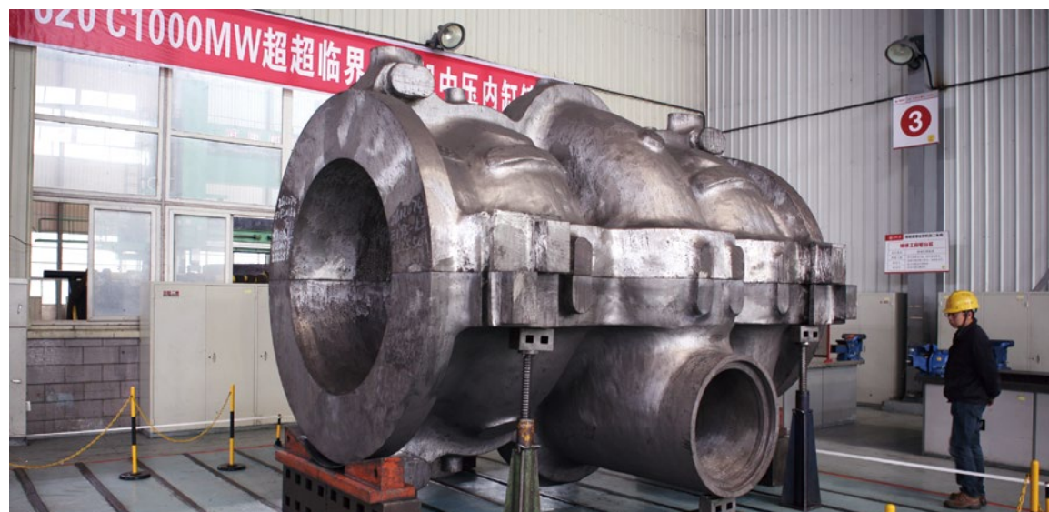
The first 620°C 1000MW ultra supercritical steam turbine cylinder casting in the world produced by China Erzhong and Shanghai Electric Group Company Limited
