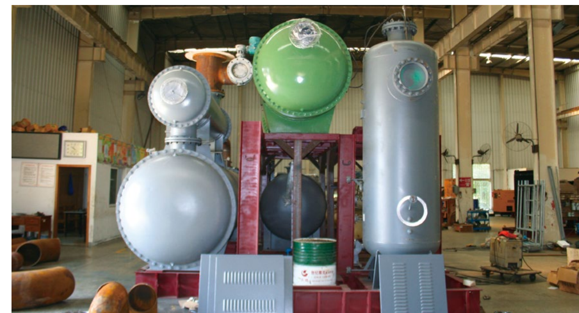
China's first low temperature waste heat recovery power generation system sample machine based on organic rankine cycle (ORC) jointly developed by CMEC and other enterprises
