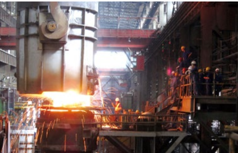
China Erzhong successfully cast a 600-ton steel ingot
