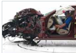
The condition of a Genesis after a small overlap crash test by the IIHS — the impact damaged the front part of the vehicle, but it is well distributed and there is no damage evident in the driver’s compartment, showing how this model ensures driver safety.
