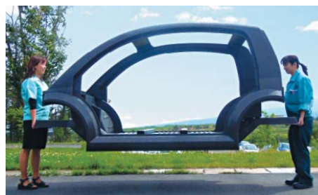
Body structure of a concept car that uses CFRP
