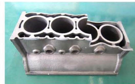
Small gas cylinder for extra-thin anti-sintering sand core casting
