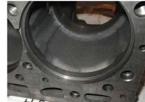
Immersion in neutral rust remover to remove rust in the internal cavity
