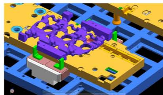
Schematic diagram of modified frameless water jacket core robot gripping techniques
