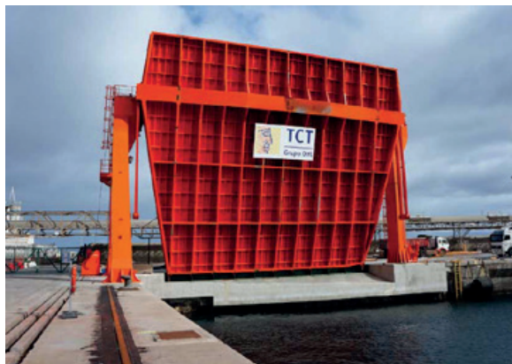
Innovative 20x25 m foldable ramp for Ro-Ro traffic with a service load of 180 tons.
