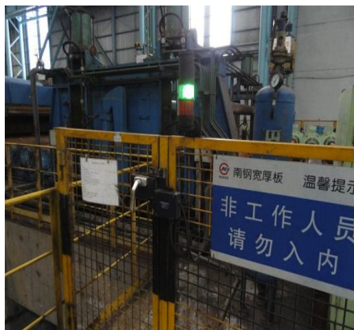
△ Case of potential problem rectification: rotating equipment area isolated and equipped with alarm interlocking device
