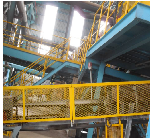
△ Case of potential problem rectification: safety protective net and supporting roller added for belt conveyer
