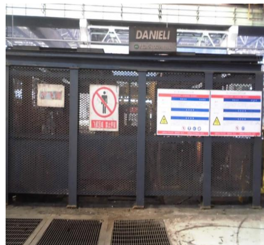
△ Case of potential problem rectification: rotating equipment area isolated and equipped with alarm interlocking device
