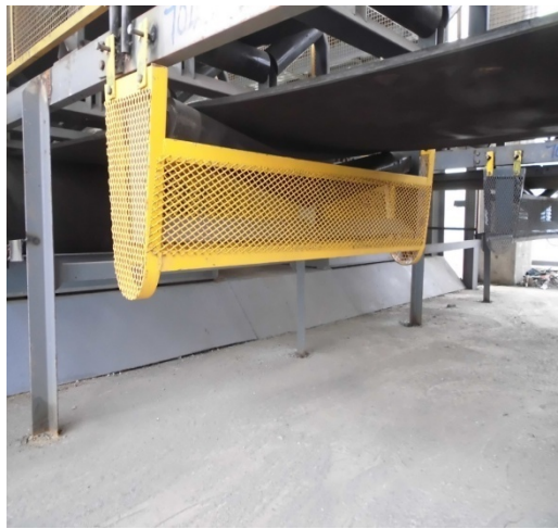
△ Case of potential problem rectification: safety protective net and supporting roller added for belt conveyer
