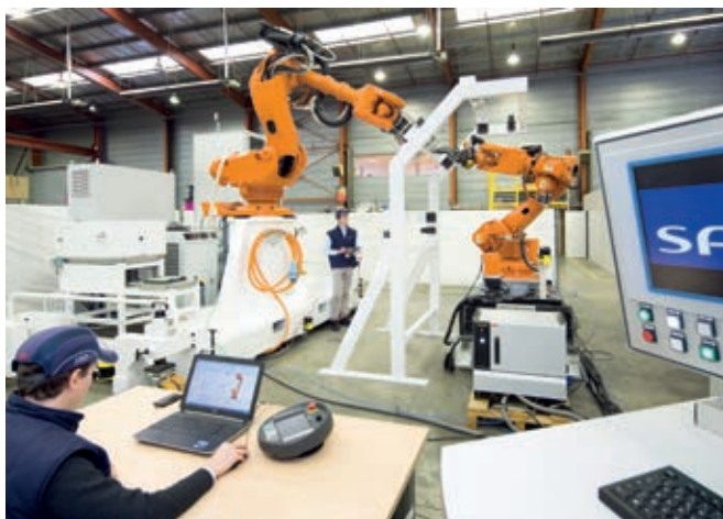
FRANCE – FXR-DAHER SOCATO: design and production of drilling/riveting module integrated on robot arm, for assembling the fuselage panels of the F5X.
