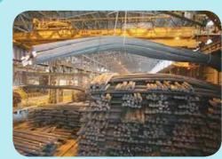
Reinforcing steel is a steel bar with ribs, commonly used in reinforcing concrete buildings. It was produced as an alternative to plain bar and substituted it in time.
