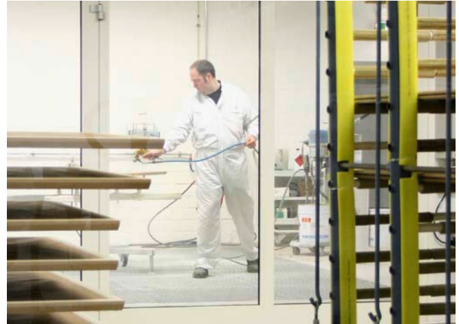
Efficient and sophisticated varnishing: by automatically mixing the varnish, applying underfloor suction and additional heat recovery, Wilkhahn makes top-quality conference and standalone tables that comply with high health-and-safety and environmental standards.
