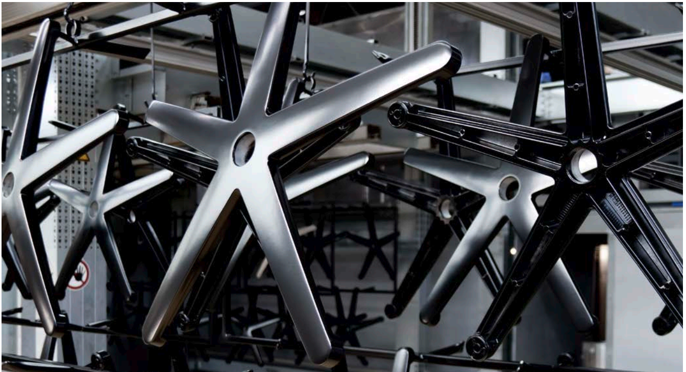
The powder varnishes used by Wilkhahn are practically free of solvents and heavy metals and come in colours to suit customer preferences.
