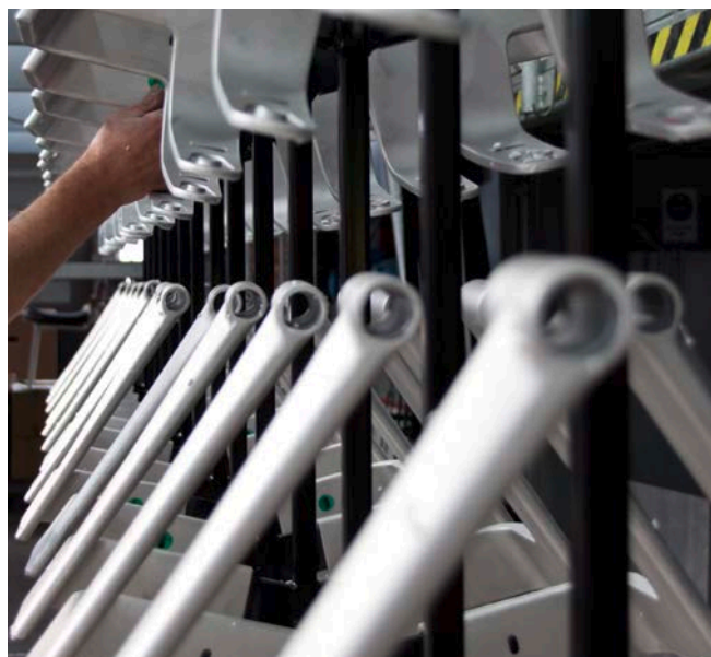
Each part is checked to ensure the surface and other quality features are perfect before the powder varnish is applied.
