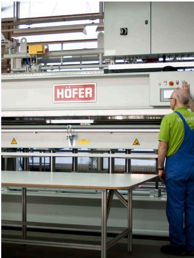
Eco-friendly table manufacture at Wilkhahn: During pressing, the water which has been heated previously in a climate-neutral manner, ensures energy-efficient and lasting bonding of adhesives.
