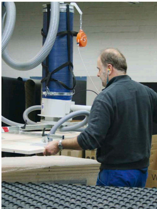
Pneumatic lifting equipment at Wilkhahn helps our employees to move table tops. This systematic support when lifting and carrying objects prevents back complaints.
